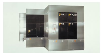
LCD lithography equipment released for sale in 2002
