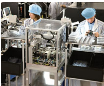
Canon's "man-machine cell" production integrates automated equipment into the cell production system. (Nagasaki Canon Inc.)
