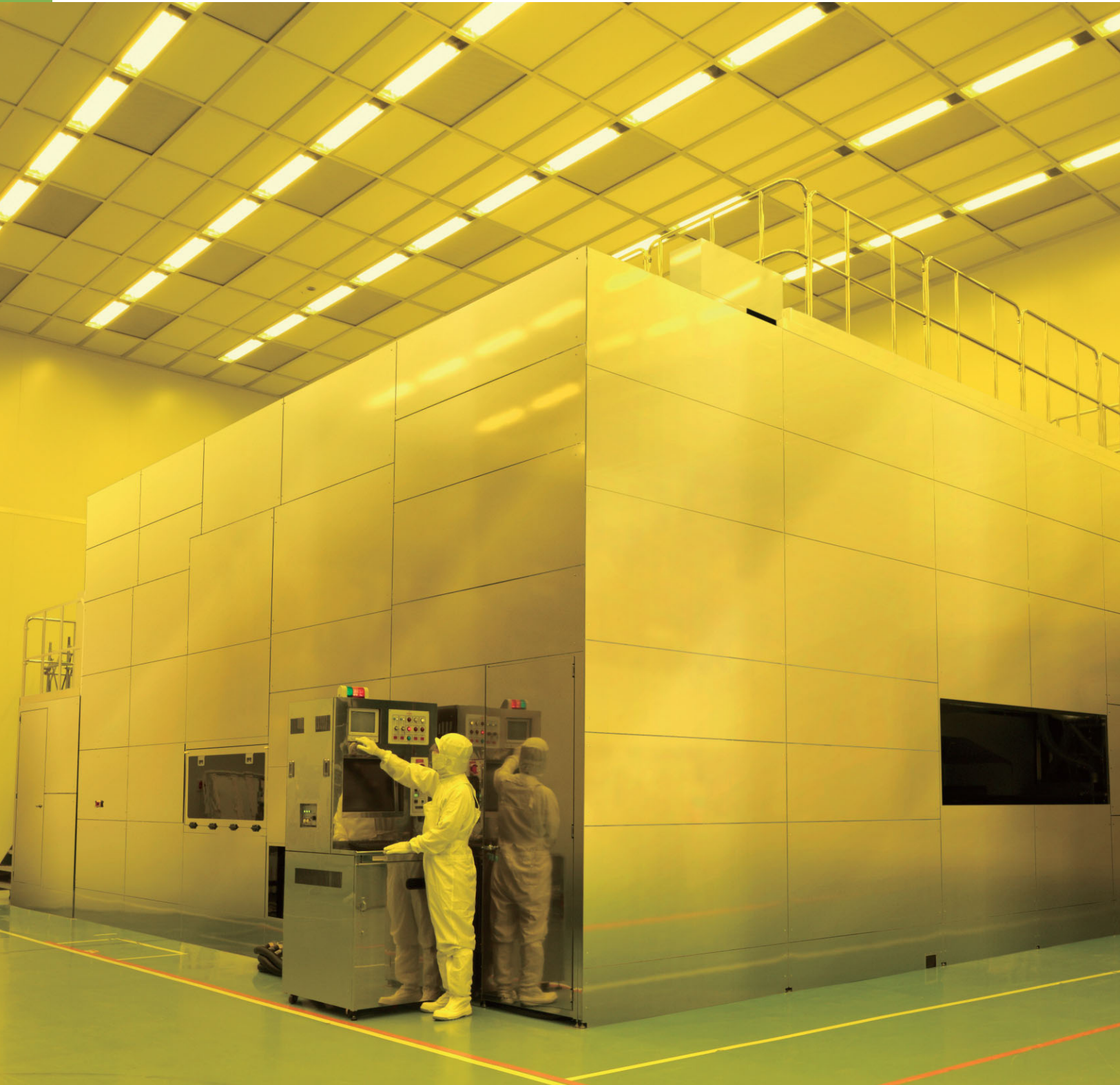
Photo: Measuring 9.0 m in width, 11.6 m in depth and 5.8 m in height, and weighing approximately 100 tons, Canon's LCD lithography equipment can accommodate eighth-generation glass substrate sizes. Canon is currently undertaking technological development for lithography equipment to support substrate sizes of 10th- and future generations, achieve a higher resolution and realize compatibility with organic light-emitting diode devices and displays.
