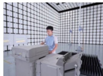
EMI measurement of products in a semi-anechoic chamber
