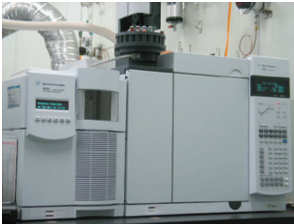
Gas chromatograph mass spectrometer used to measure chemical substances emitted from products
